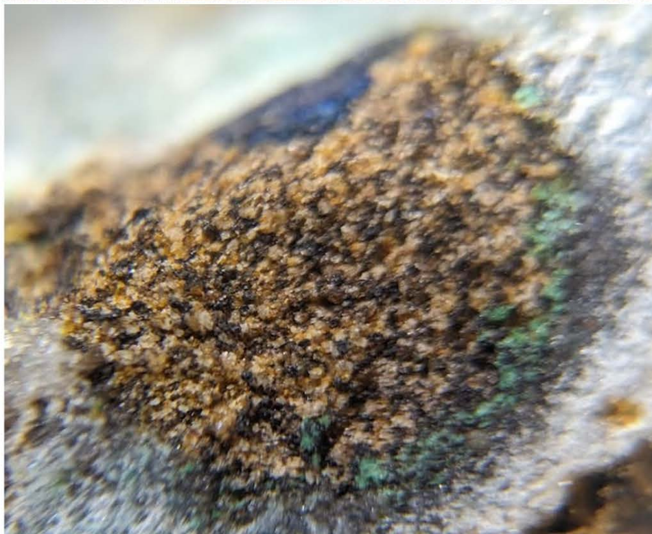
Figure 4. Two photos from channel 869. The top photo illustrates the strong surface leaching of copper sulfide. The white leached surface holds 0.04 % Cu (pxrf) and the partially leached greenish core with copper oxides holds 1.7 % Cu (pxrf).
