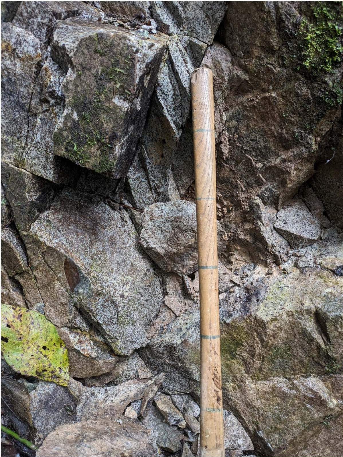
Figure 3. Photo from channel Ch869 uncut assaying 13.4 m @ 1.4% Cu and 29 g/t Ag. Including 5.8m @ 3.1% Cu and 65 g/t Ag. The host rock is a reduced white sandstone with concretions of iron oxides replacing iron rich carbonates. The scale of the hammer is 10cm intervals.
